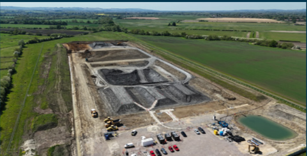
Image: Costain An image of the clay compaction trial site from May 2025 in Abingdon, Oxfordshire, to inform the design of SESRO.
